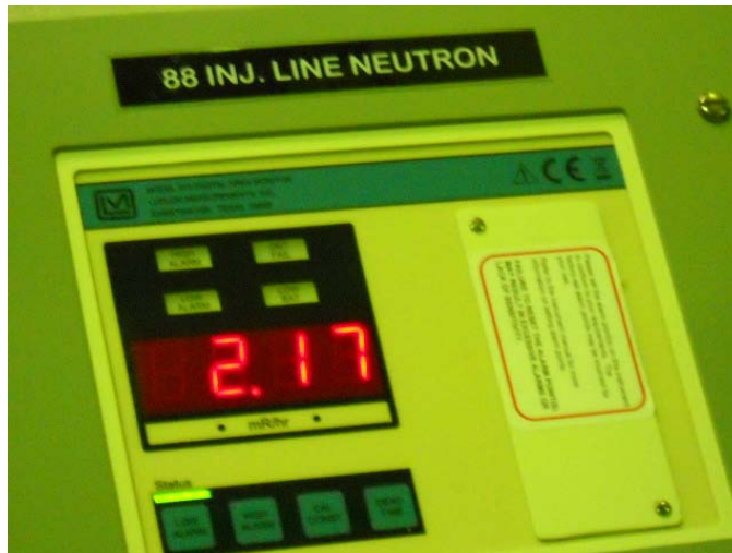
FIG. 9. Secondary radiation levels of 2 – 3 mRem/hr were measured at the injection line above the K150 cyclotron while 14 \mu A of 30 MeV protons were stopped on the exit Faraday cup of the K150 cyclotron. H - ions accelerated to 30 MeV were stripped to protons at the extraction radius .
