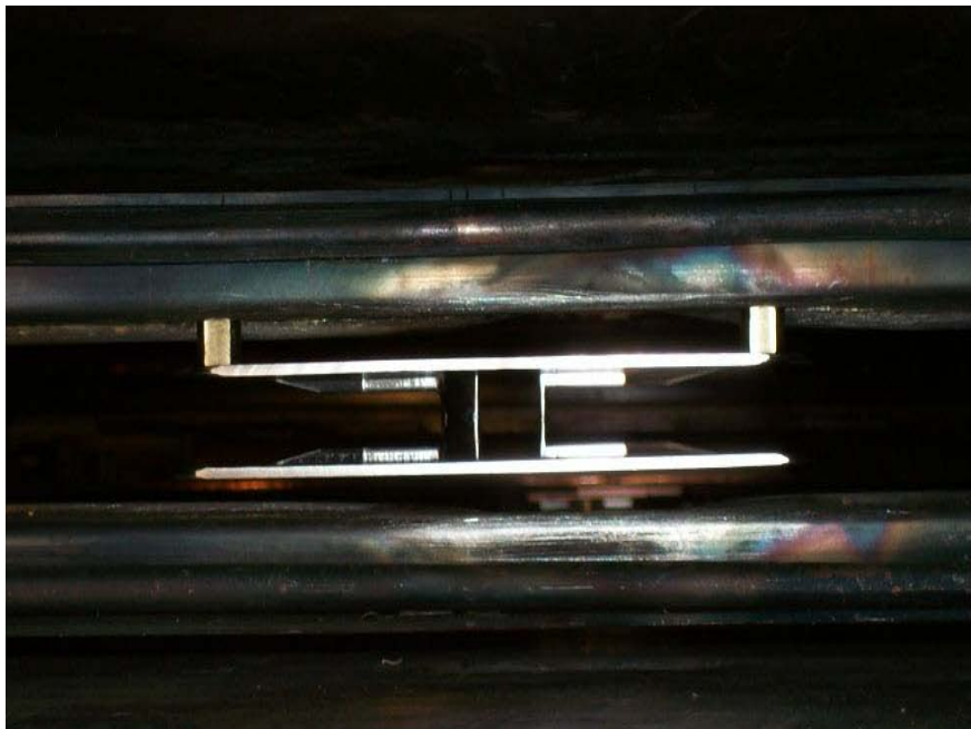
FIG. 3. Photo of the dummy dee side batwing after the installation.
